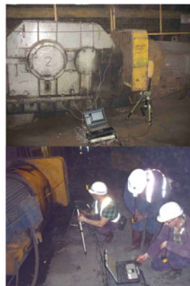
Fig. 3 Maintenance inspection for conveyor gearbox—vibration measurement using Diag Manager system
